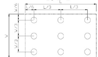
L max: The measured Maximum luminance of all measurement position.
